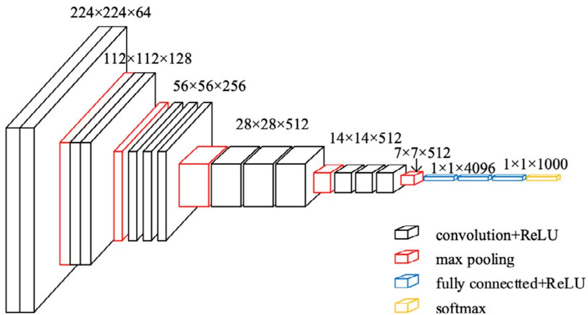
**Figure 1.** Structure of vgg-16 network model
