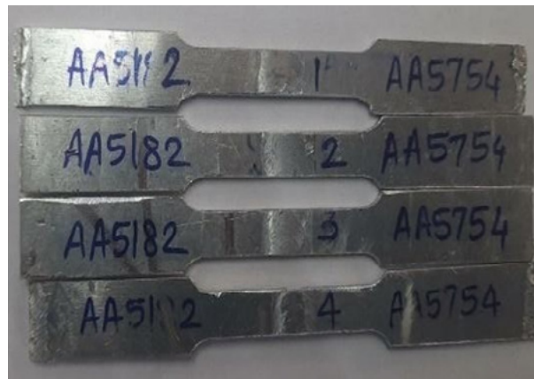
Figure 5. Tensile test specimen of TWB
