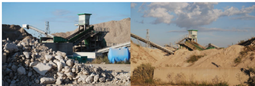
Production of recycled aggregates with different particle sizes in the Ecologica 2000 plant in Rome.
