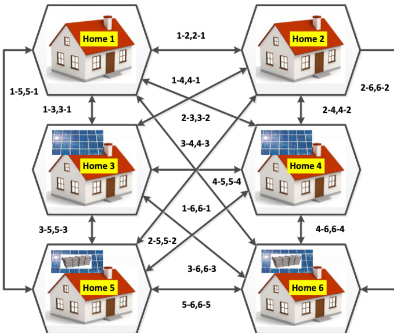
Figure 5. Decentralized Cooperative Community Microgrid Design.
